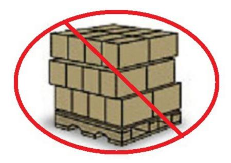
Interlocked stacking patterns can reduce stacking strength by up to 50%.
