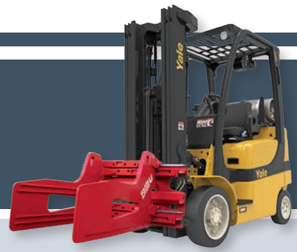
▲ The Veracitor® VX series lift truck is designed for medium- to heavy-duty applications. Here a GC050VX is equipped with a Bolzoni bale clamp.
