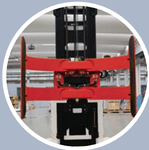
▲ AGVs - Automated Guided Vehicles, are customized, fully-automated, driverless vehicles for continuous 24/7 operation, capable of transporting pallets, boxes, reels and other products throughout warehouses and production plants. In cooperation with main AGV producers, Bolzoni has developed a range of attachments equipped with specific sensors managed directly by the AGV control unit.
